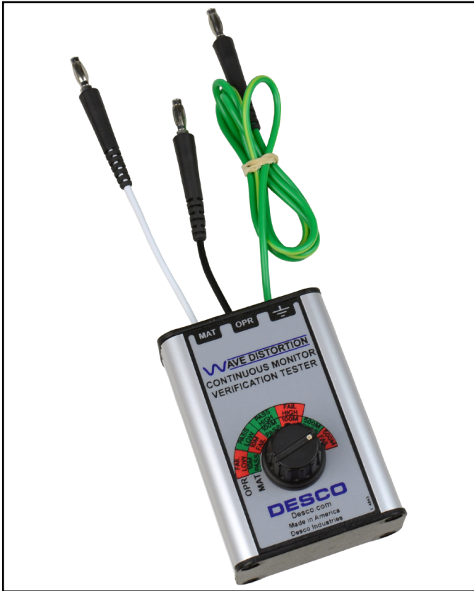
Figure 1. Desco 98221 Wave Distortion Monitor Verification Tester
